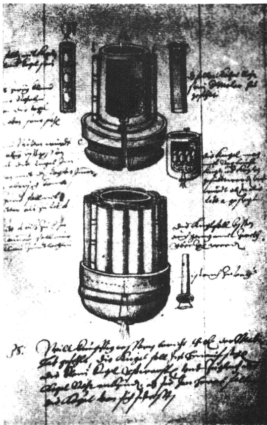
Figure 7b & 7c Sketch by Sebisch of rocket battery, about 1600 (left); and of his two-stage rocket (right) [31].
