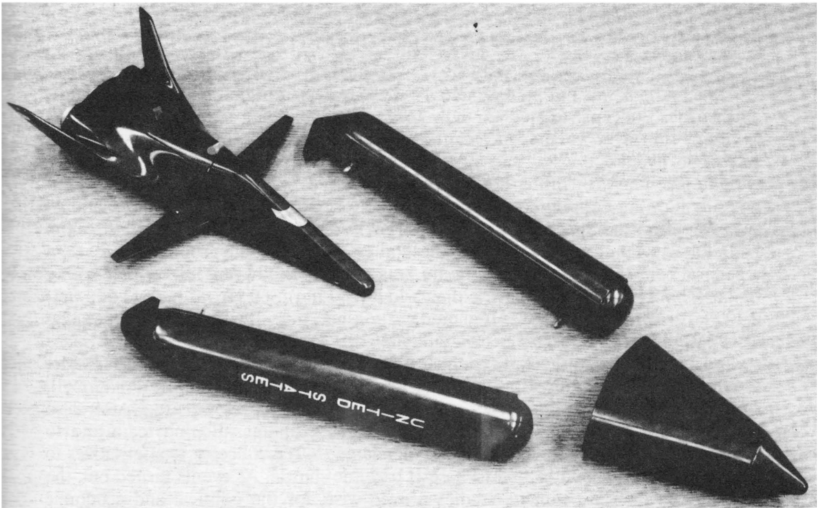
Figure 9 Lockheed "stage-and-a-half" shuttle concept, utilizing a variable geometry lifting body orbiter with flanking external fuel tanks and nose cap 1969.
