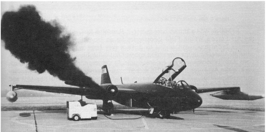
Figure 4 Top (a) Modifications to a RB-57 to use liquid hydrogen-oxygen in one engine (NACA Lewis Research Center, circa 1957). Bottom (b) The modified RB-57 with liquid hydrogen tank in right pod. The smoke is normal for starting the unmodified engine.
