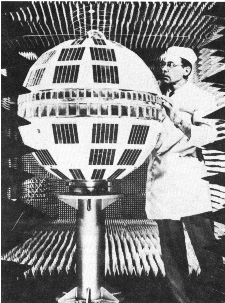
Figure 2 The Telstar satellite, developed and built by the American Telephone and Telegraphy Company.
