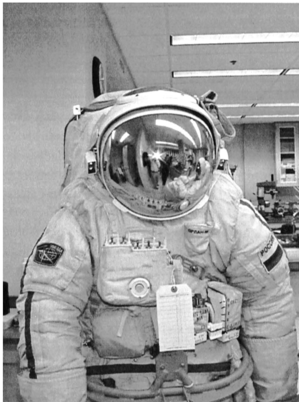
Figure 4: The Orlan-M spacesuit for extravehicular activities undergoing testing at the NASA Johnson Space Center (Photo Courtesy of NASA).
