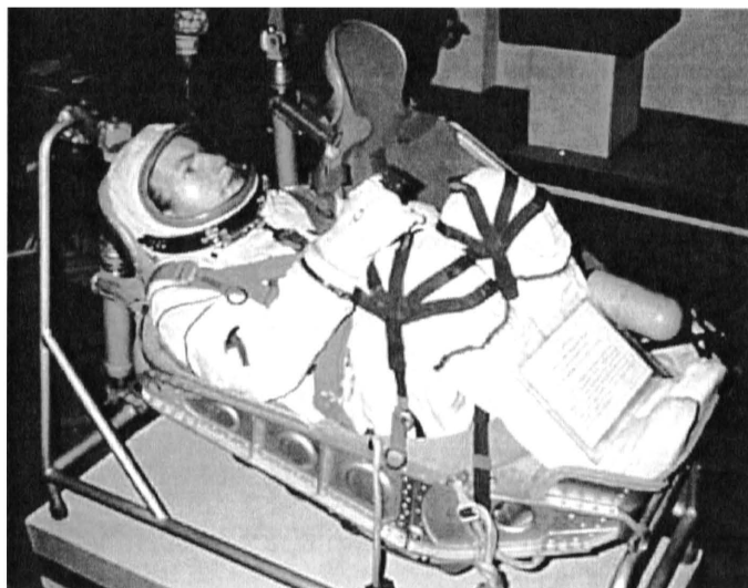
Figure 3: The Sokol SK-2 spacesuit in the Kazbek-U couch from the Soyuz spacecraft, on display at the Zvezda Museum (Courtesy of the Smithsonian Institution).
