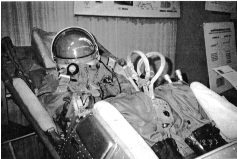
Figure 1: The SK-1 spacesuit in the Vostok ejection seat, shown on display at the Zvezda Museum outside of Moscow (Courtesy of the Smithsonian Institution).
