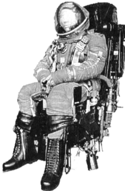
Figure 5: The Strizh full-pressure suit was developed for the Buran program (Courtesy of Zvezda).
