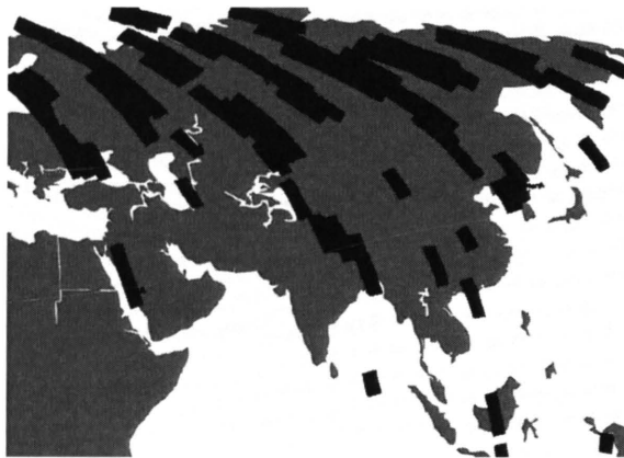
Figure 17–10: This image illustrates the areas recorded by a KH-4A over a four-day mission, specifically mission 1017. 16
