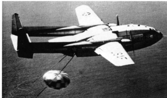
Figure 17-8: A C-119 "Flying Boxcar" catching a CORONA film bucket near Hawaii. 13
