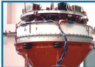
Equipment Bay vibration test
