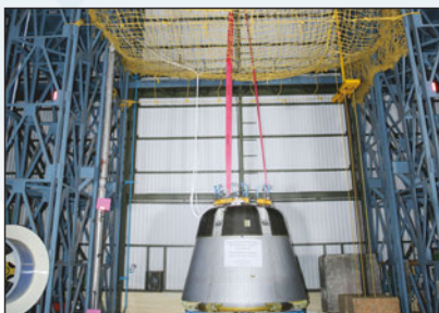
Apex Cover separation test
