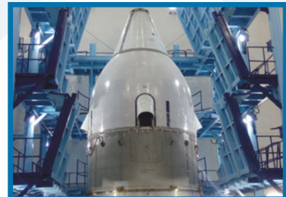
CES Ground Resonance Test
