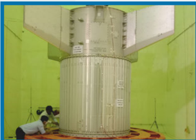
Integrated Base Shroud Acoustic test
