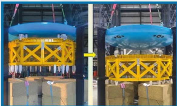
Service Module separation test
