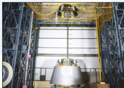
Apex Cover separation test
