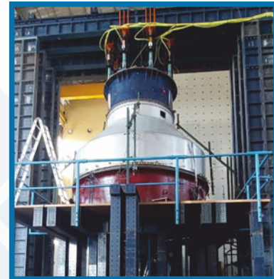
Integrated structural test of Interface Adapters
