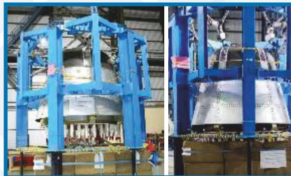
Crew Escape System separation test
