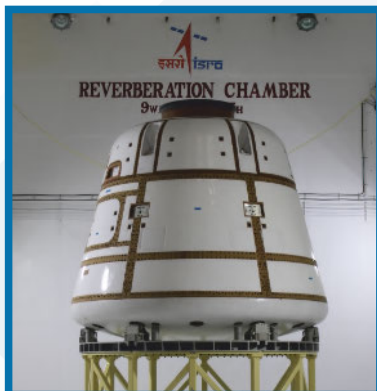
Crew Module Acoustic Test at ISITE, URSC
