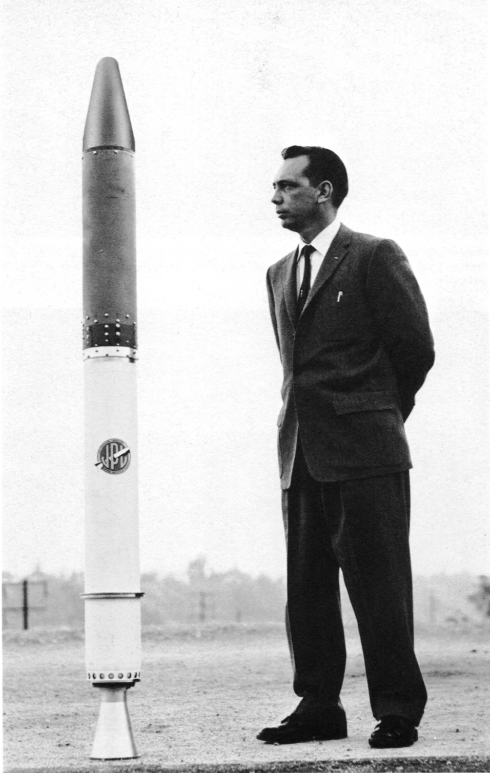
The 18-pound Explorer I payload with its motor (shown here with Explorer Project Manager Jack E. Froehlich) was 80 inches long and 6 inches in diameter. On January 31, 1958, Explorer I was successfully injected into an elliptical orbit ranging from 220 to 1563 miles above the earth. Although no longer transmitting a signal, the spacecraft is still in orbit today.
