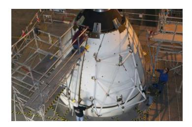
Technicians attached the fourth and final Ogive panel on the Orion ground test vehicle in Vehicle Assembly Building high bay 4 at NASA's Kennedy Space Center in Florida. The Ogive panels enclose and protect the Orion spacecraft and attach to the Launch Abort System. The test vehicle is being used by Ground Systems Development & Operations (GSDO) for pathfinding operations, including simulated manufacturing, assembly and stacking procedures.
