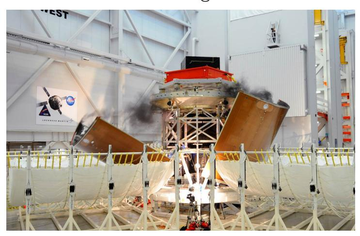
At the Lockheed Martin facility in Sunnyvale, Calif., the team conducted the first in a series of tests to determine if the Orion spacecraft can successfully jettison its protective fairings, or covers, during its ride to space. During the first of these tests, two of the three fairing panels separated as planned, but a third did not.
