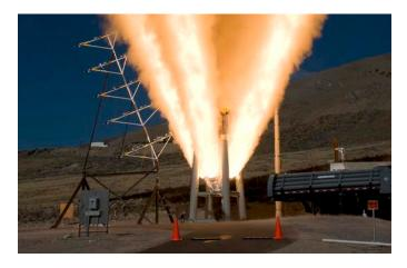
Orbital ATK successfully completed its Critical Design Review (CDR) with Lockheed Martin and NASA for the Orion launch abort motor on Aug. 6. The abort motor is a major part of the Orion Launch Abort System (LAS), which will help ensure the safety of astronauts who launch on missions to explore deep space aboard NASA's new, heavy-lift Space Launch System (SLS).
