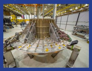
Pieces of the Exploration Mission-1 Orion spacecraft being prepped for welding at NASA's Michoud Assembly Facility.
