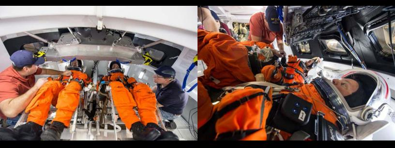
Engineers at NASA's Johnson Space Center in Houston are evaluating how crews inside a mockup of the Orion spacecraft interact with the rotational hand controller and cursor control device while inside their spacesuits. The controllers are used to operate Orion's displays and control system, which the crew will use to maneuver the spacecraft.
