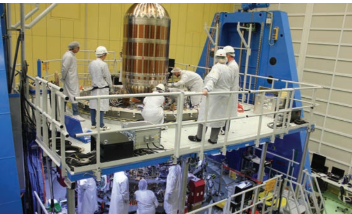
Technicians at the Airbus facility in Bremen, Germany install the fuel tanks on the European Service Module for Exploration Mission-1.
