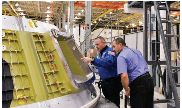
Astronaut Butch Wilmore reviews the welding progress on Orion's Exploration Mission-2 crew module pressure vessel at NASA's Michoud Assembly Facility in New Orleans, Louisiana.
