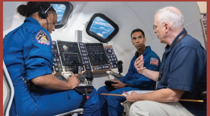
The Orion Rapid Prototype Lab (RPL) team recently conducted the fifth in a series of "mini-sims" with NASA astronauts and a small team of flight controllers. The team designed and executed complex and innovative simulations of the newly prototyped Orion crew on-orbit burn display formats and electronic procedures. The RPL team gained valuable experience using these displays and procedures in a more realistic scenario with crew members and the ground control team. These evaluations will help to validate or identify areas needing updates to ensure key changes can be made earlier and more economically in the software development cycle. The team consisted of members from Aerospace Applications North America, Barrios Technology, Ames Research Center and interns from NASA and SGT.
