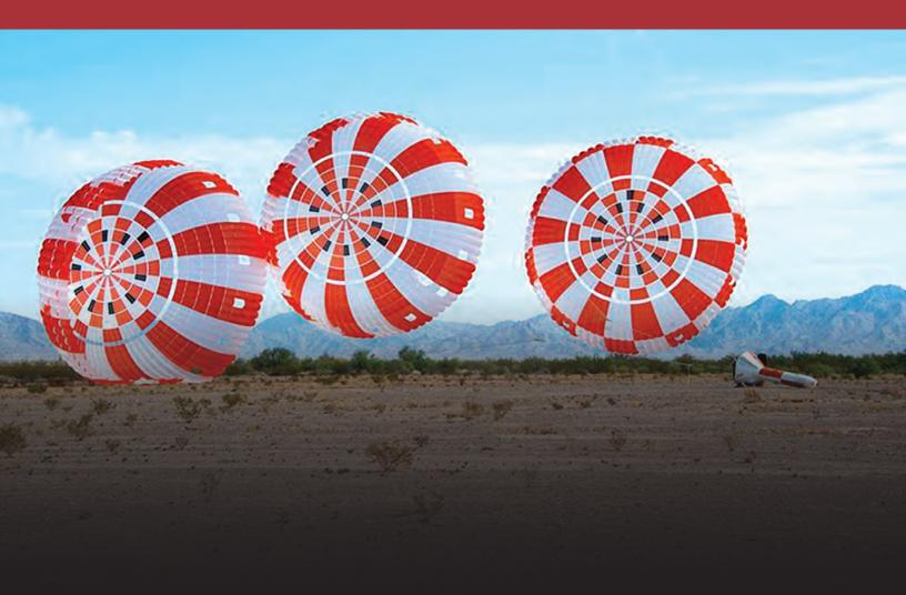
The parachute system for Orion, America's spacecraft that will carry humans to deep space, deployed as planned after being dropped from an altitude of 6.6 miles on July 12 at the U.S. Army Proving Ground in Yuma, Arizona. Data from the successful seventh drop in a series of eight qualification tests will help NASA engineers certify Orion's parachutes for missions with astronauts.
