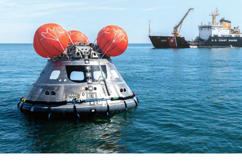
Engineers completed two key tests the week of March 18 to help ensure NASA's Orion spacecraft is ready from liftoff to splashdown for missions to the Moon. Teams successfully tested one of the motors on Orion's Launch Abort System responsible for taking the crew to safety in an emergency during launch, and completed testing at sea for the qualification of the system used to upright Orion after it lands in the ocean.
