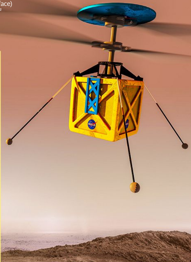
One prototype of the Mars helicopter used PVC tracking balls and cameras to fly itself.
