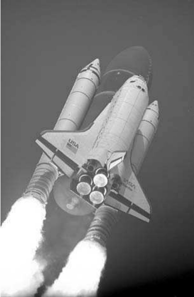
Figure 9.2: The space shuttle Atlantis climbs away from Kennedy Space Center on the STS-45 mission of March 1992. The shuttle is powered, at this stage of its flight, by the orbiter's three main engines (arranged in a triangle below the tail fin) and the two large, white solid rocket boosters flanking the fuel tank beneath the orbiter. The two smaller engines of the orbital maneuvering system (OMS) are contained in the bulges flanking the tail fin. Their exhaust nozzles are visible to either side of the uppermost main engine. Courtesy of NASA Kennedy Space Center, image number 92PC-0644.
