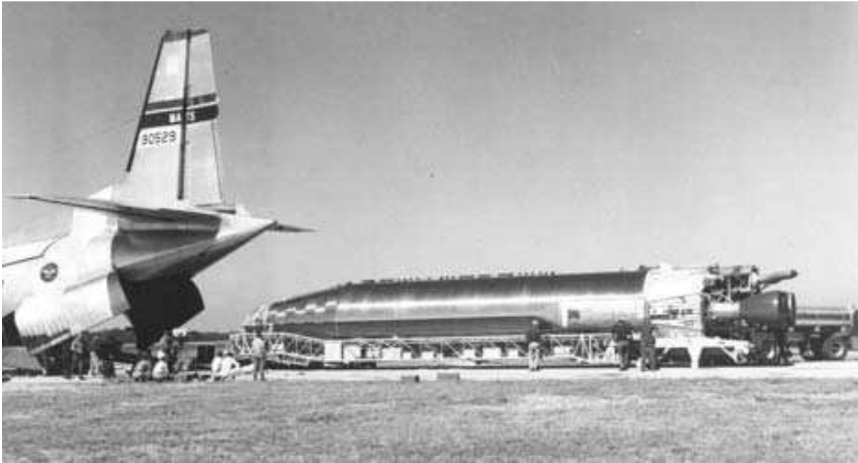
Figure 6.2: NASA employees watch as an Atlas missile is unloaded from a military transport in 1961. The two men standing near the tail of the missile give an idea of its size. Atlas, the first American ICBM, was a major technological step beyond earlier missiles and the first U.S. launch vehicle capable of putting a manned spacecraft in orbit. It launched John Glenn's three-orbit flight in February 1962, and the three Project Mercury flights that followed it. Courtesy of NASA Kennedy Space Center, image number GroundAtlas.
