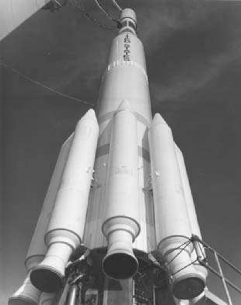
Figure 6.4: A Delta launch vehicle, augmented by strap-on boosters and carrying the Nimbus 5 weather satellite, waits on its launch pad at Cape Canaveral in 1972. The Delta, which evolved from the Thor-Able pictured in Figure 6.3, has been the most successful of all U.S. launch vehicles. An updated version, the Delta II, is still in service. Courtesy of NASA Headquarters, image number Nimbus-Delta.
