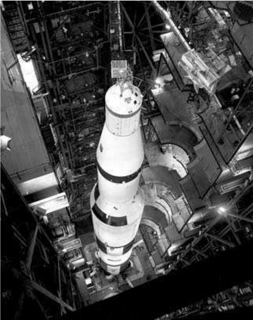
Figure 7.2: A complete Saturn-Apollo “stack,” photographed from the upper floors of the Vehicle Assembly in 1967. This particular vehicle is AS-501, which was used for the Apollo 4 mission (the first all-up test of the Saturn launch vehicle and Apollo spacecraft) in November 1967. Courtesy of NASA Kennedy Space Center, image number 67P-0208.
