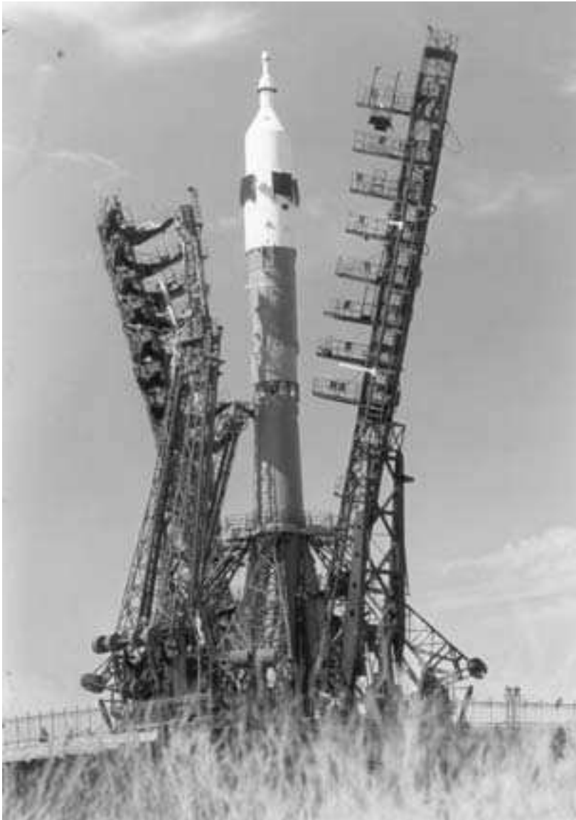
Figure 9.1: A Soyuz-U launch vehicle on the launch pad at Baikonur, Kazakhstan, preparing to launch the Soyuz spacecraft that would take part in the Apollo-Soyuz orbital rendezvous of 1975. A descendent of the R-7 missile, the Soyuz-U is the most widely used and most reliable manned launch vehicle in history. Courtesy of NASA Headquarters, image number 75-HC-606.
