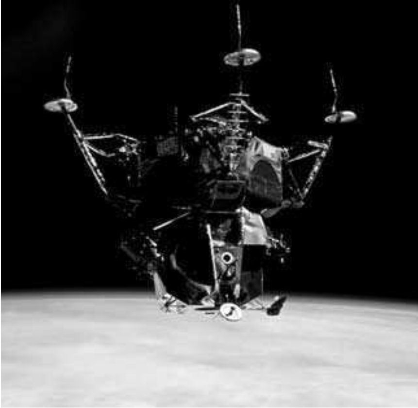
Figure 7.3: The first orbital test flight of the Apollo LM, part of the Apollo 9 mission of January 1969. Designed to fly only in airless space, the LM had no need for streamlining or equipment for landing on Earth. Here it is flying “upside down,” with its docking port at the bottom of the photograph, toward the Earth’s surface, and its legs (extended in landing position) at the top. Photograph by Apollo 9 command module pilot David Scott. Courtesy of NASA Johnson Spaceflight Center, image number AS9-21-3212.
