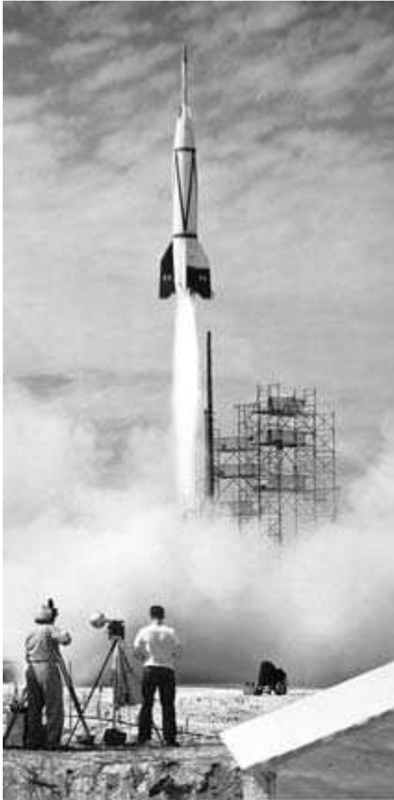
Figure 5.1: A converted V-2 with a WAC Corporal upper stage, part of Project Bumper, lifts off from the Army Missile Range at Cape Canaveral, Florida, on July 24, 1950—the first launch from what would become Kennedy Space Center. Courtesy of NASA Kennedy Space Center, image number 66P-0631.
