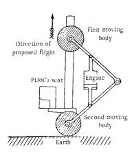
FIGURE 78. Flight with the help of movement of masses
