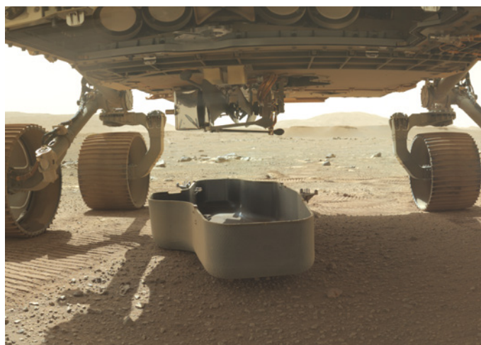
▲ SHIELDS DOWN Perseverance dropped the debris shield protecting Ingenuity on March 21, 2021, and peeked under itself with the WATSON camera on its robotic arm to take this image.
