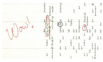
▲ **"WOW!**" The Big Ear Radio Observatory recorded incoming signals' brightness first using numbers and then, if the signal was bright enough, in letters. The letter "U" indicates a signal 30 times the background noise level; the signal as a whole lasted 72 seconds.
