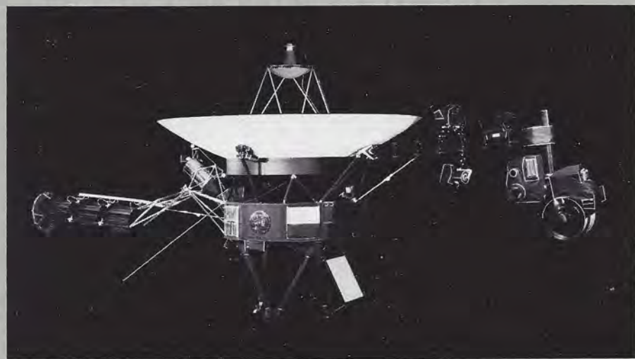
ABOVE: Voyager's 3.7-meter-wide antenna dominates the appearance of the spacecraft.
