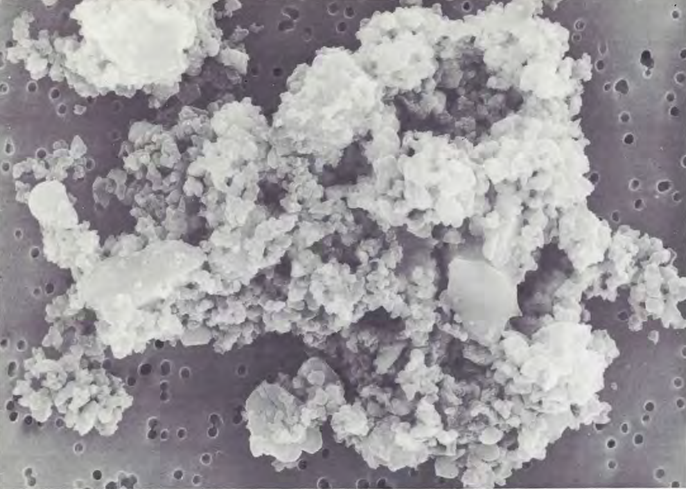
Collected by a high-flying U-2 aircraft, this tiny particle of extraterrestrial dust, only a few hundredths of a millimeter across, displays an aggregate of even tinier crystals.
