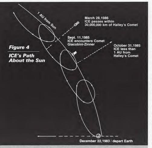
FIGURE 4: As it travels about the Sun, ICE will encounter Comet Giacobini-Zinner on September 11, 1985. Also, as shown in this chart, ICE will twice pass fairly close to Halley's Comet. The trajectory here appears to have a looping motion because it is plotted with respect to a fixed Sun-Earth line. (An Astronomical Unit, or AU, is the average distance from the Sun to Earth, about 150 million kilometers.)
