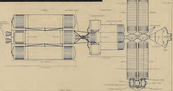
The <u>Mars One</u> Main Ship is a modular structure, consisting mostly of fuel tanks. The crew will ride in the habitability (HAB) modules, each 15.2 meters (50 feet) in length and 4.3 meters (14 feet) in diameter. Tunnels connect the HAB modules with the laboratory and storage modules, and with the Mars Excursion Module (MEM). Drawing: Paul Hudson
