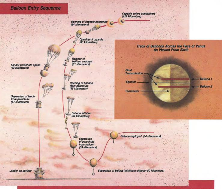
ABOVE: Vega's deployment of the balloons and landers at Venus required many steps that were performed at specific altitudes to prepare the probes for their missions. INSET: The Vega balloons entered Venus' atmosphere on the nightside and floated across the terminator (the boundary between day and night) well into the dayside. Illustrations: S.A. Smith
