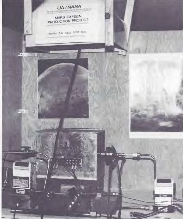
This unassuming apparatus, built at the Space Engineering Research Center at the University of Arizona, is the experimental prototype of a device that may someday produce oxygen from carbon dioxide on Mars. The ability to use extraterrestrial materials to fuel missions from Earth may help make the human exploration of Mars and the Moon affordable.
