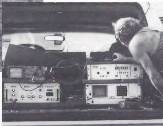
LEFT: Both the SNAKE and the gondola suspended beneath the balloon carried instruments to measure our apparatus' performance. The back of one of our four-wheel-drive trucks was turned into a mobile laboratory to monitor the incoming data. We compiled information on the system's speed, its dynamic state and the inclination of the tethers as it moved, the wind speed relative to the balloon, gas temperature within the balloon and the temperature of the surrounding air. All this will help to predict how the balloon and SNAKE will perform on Mars.
