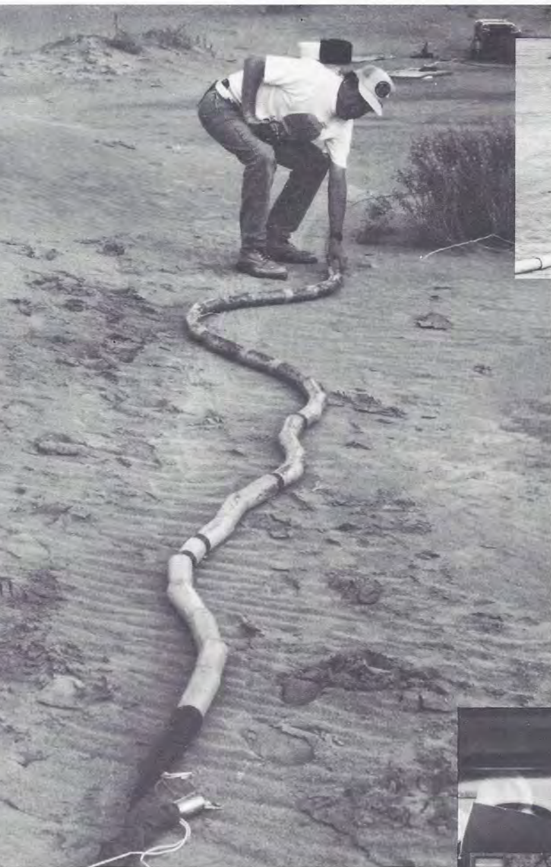
ABOVE: The SNAKE waits patiently as the balloon is readied, disturbed only when Society Executive Director Lou Friedman tweaks its tail. The "nested Dixie cup" design gives the SNAKE the flexibility to serve as a self-ballasting guide-rope for the balloon, as well as the rigidity to avoid snagging and to protect its internal instruments.
