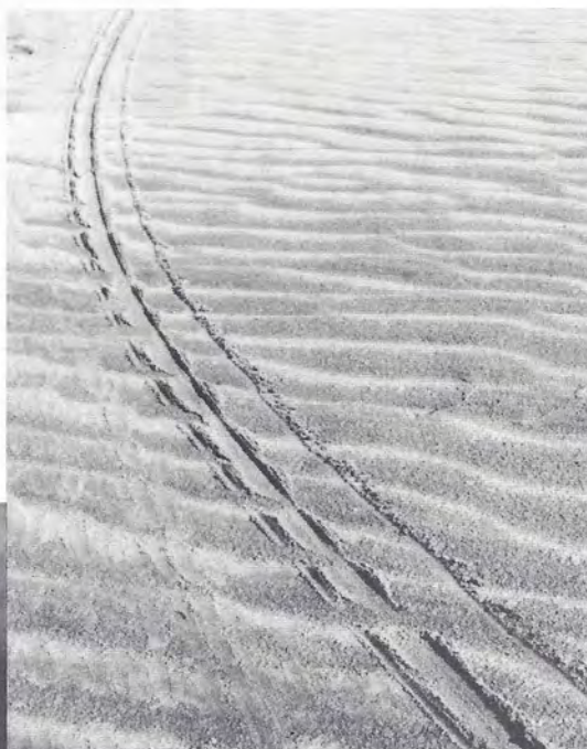
ABOVE: The SNAKE left distinctive tracks in the Mojave sand. Here its trail crosses ripples formed by wind erosion. As the fluctuating, gentle wind moved the balloon from side to side, the SNAKE rolled, leaving wide, sinuous patterns on the dunes. The SNAKE tracks were especially visible because the previous night's rain had darkened the dune surfaces.
