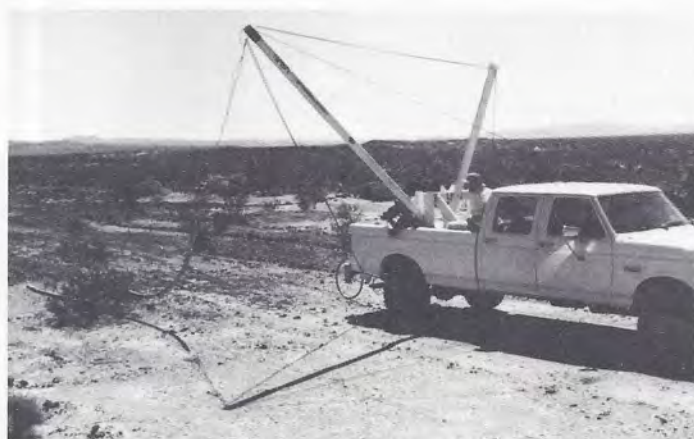
ABOVE: Tests early in the summer involved dragging the SNAKE behind a truck and monitoring performance. Here it encounters scrub brush, an obstacle unlikely to be encountered (unfortunately) on Mars. Photo: Lazlo Keszthelyi
