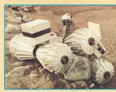
ABOVE: The minirover proves that small boulders are no problem as it steps and rolls over this obstacle. This design is a "wheel-walker" and has six conical wheels capable of moving independently in a sort of crawling motion, thus combining elements of both walker and wheeled rover designs.
