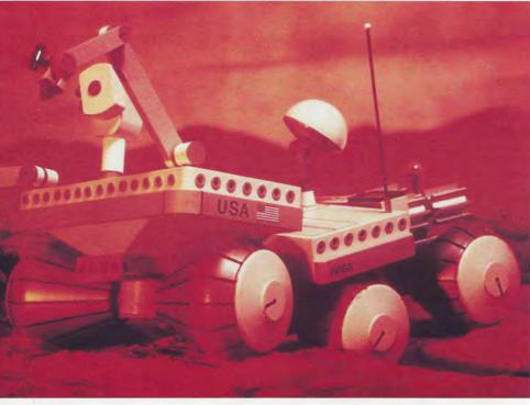
of Ball Aerospace has studied an alternative concept, in which a minirover with a simple camera constantly scans the horizon and moves to the highest elevation it sees, repeating this action until it reaches a vantage point suitable for a panoramic view. Minirovers obtaining such panoramic views might compete with large, high-resolution imagers or even large multipurpose rovers for surveying possible human landing sites.
