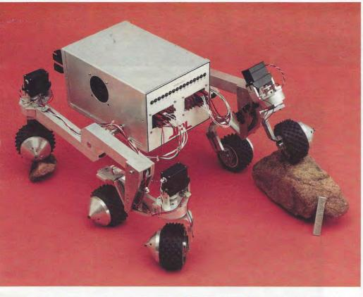
LEFT: The prototype Rocker Bogie is able to scale obstacles more than twice a wheel diameter in size (its wheels are fiveeighths the size of the Bickler pantograph's). "Rocky" has had a computer brain added and is now being used in field tests as a minirover.
