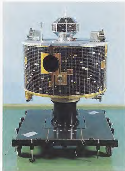
Called Muses-A at its launch in January 1990 and later re-named Hiten, this spacecraft carried the small subsatellite Hagoromo to the Moon, where the smaller craft's transmitter failed. Hiten executed a series of lunar swing-bys in 1990 and Earth aerobraking demonstrations in 1991. Then, following a path discovered by the author and James Miller, the spacecraft undertook a new mission to orbit the Moon.
