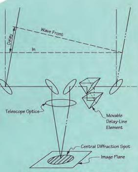
In a Michelson interferometer, the two beams of light alternately interfere destructively or constructively, giving fringes (bright and dark bands) in the image plane. The path lengths are equalized by delay line optics, giving a very precise measurement of the direction to the source of the waves. Diagram reprinted from TOPS
