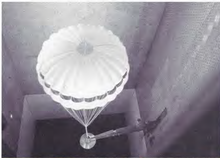
A scale model of the Huygens probe, fitted with scaled parachutes, was recently tested in the transonic wind tunnel at Arnold Air Force Base in Tennessee. The results will be used to verify that the parachute and probe combination will work as designed at Titan. Photograph: Arnold Engineering Development Center
