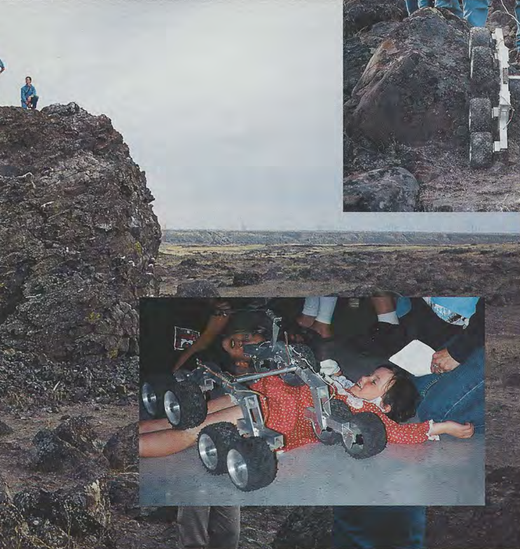
Above: The Scabland proved a challenging test site for an eight-wheeled prototype of the Sojourner rover that Pathfinder will carry to Mars. Any Mars rover's primary goal will be to explore without getting stuck; the rovers are off-road vehicles par excellence. The strange, multiwheeled designs are engineers' solutions to navigating almost any terrain the rovers might encounter.
