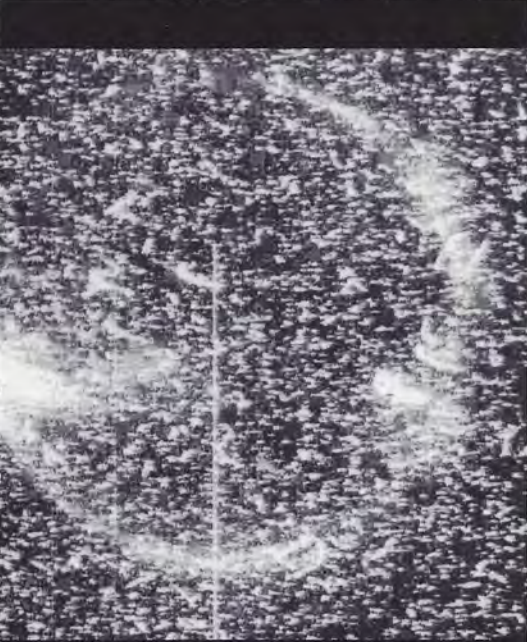
Io in eclipse by Jupiter does not present a pretty picture. However, this 6.3 second exposure does show the dramatic effects of magnetospheric radiation on Galileo's cameras. Because of the long exposure, the glowing volcanoes appear as shapes resembling check marks, as do stars outside the circle that is Io. But the rest of the glitches are due to radiation. During the coming close encounters with Io, Galileo will be exposed to even more intense radiation, which may dominate its images.
