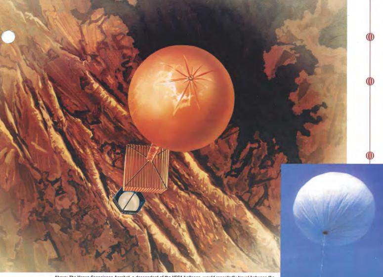
Above: The Venus Geoscience Aerobot, a descendant of the VEGA balloons, would repeatedly travel between the cool upper atmosphere, with temperatures around 0 degrees Celsius (32 degrees Fahrenheit), to the quite nasty lower atmosphere, where it would have to endure temperatures up to 460 degrees Celsius (about 860 degrees Fahrenheit). Illustration: JPL/NASA
