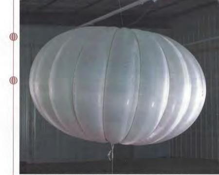
Above: NASA is testing various designs for ultra-long-duration balloons in Earth's atmosphere, and some of these superpressure designs might someday fly on Mars. This is the pumpkin design from the space agency's Wallops Flight Facility. Photo: NASA
