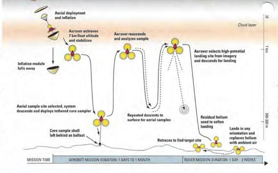
scopic data that could help unlock the secrets of the evolution of Venus. From an altitude of about 55 to 60 kilometers (roughly, 35 miles), moving rapidly with the zonal winds, an aerobot would deploy precisely timed sondes into the surface features of highest scientific significance.
