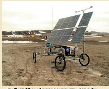
The "Hyperion" Sun-synchronous robotic rover underwent successful field trials on Devon Island in July 2001, under the leadership of David Wettergreen and Red Whittaker of Carnegie Mellon University's Robotics Institute. Navigating through rock fields and avoiding obstacles autonomously, the rover also managed its power on its own by tracking the never-setting Sun. Hyperion went on circuitous tours several kilometers in diameter and roved 24 hours a day without human intervention.
