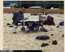
FIDO's instrument arm is deployed to examine the small rock in front of it in JPL's Mars Yard. This rock appeared much larger to the Student Navigators, who saw it through the paired hazard cameras visible at the front of the rover. Photo: ESL
