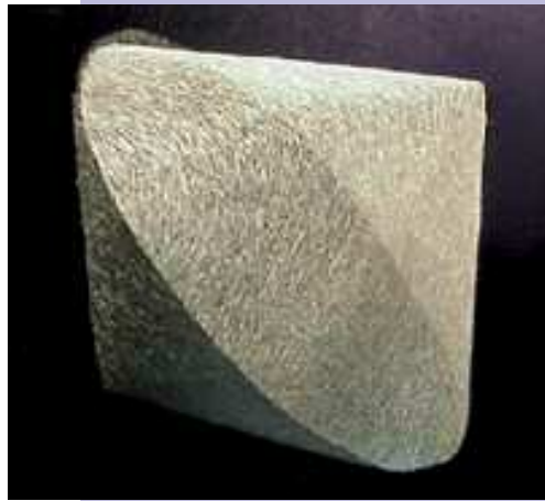
Conical sails are a natural for microwave beam-riding as they keep their shape and are easy to reposition if the beam moves off center. This model of the cone sail is about 7 centimeters (about 3 inches) wide in size.
