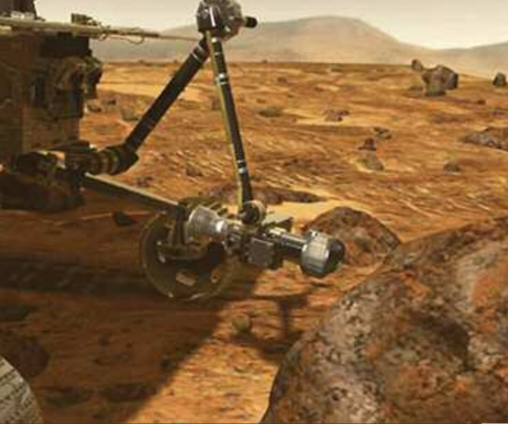
The Rock Abrasion Tool on the rover's robotic arm will spin around and grind circular patches off the surface of rocks, exposing their interiors to scrutiny by scientific instruments. Illustration: JPL/NASA
