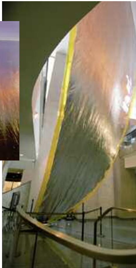
The full-size (15-meter) Cosmos 1 solar sail blade is shown deployed (right) in the lobby of New York's Rockefeller Center. The upper part, or end, of the solar sail blade is shown in the inset.
