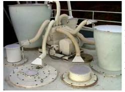
Various size feeds on top of the GBT's dish receive signals at different wavelengths. The author was relieved to see that each feed had its own snowblower. Photo: Sami Asmar
