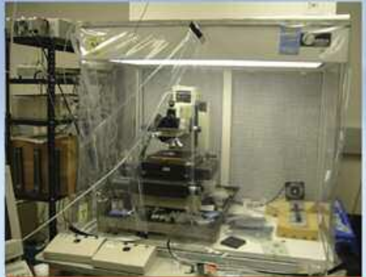
This is the automated microscope at the University of California, Berkeley (before it was moved to Johnson Space Center) that will scan the Stardust aerogel collector containing the interstellar dust samples. It will create 1.6 million "movies" to be scanned by Stardust@home participants.
