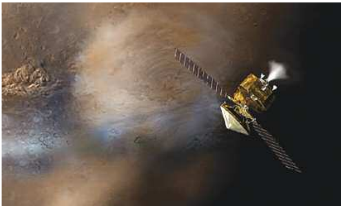
A new chapter in Mars exploration has begun. In this view, MRO fires its six main thrusters to enter Mars orbit on March 10, 2006.
