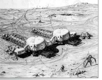
redundant systems in case of emergency or equipment failures. Each HAB has an attached, inflatable greenhouse, airlocks, and rock sample racks accessible by robot arms, and a small airlock for hands-on examination. In a nearby crater, a small nuclear generator provides initial electrical energy.
