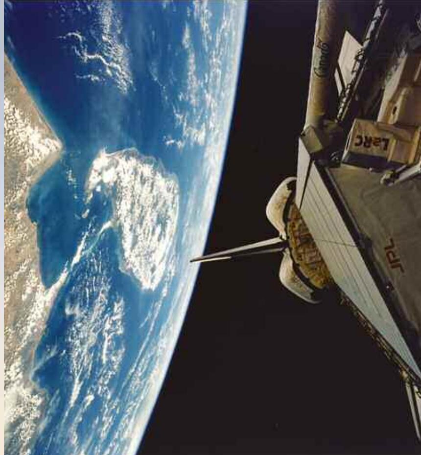
The Space Radar Lab (SRL) rests in Endeavour's payload bay as the shuttle soars 224 kilometers (about 139 miles) above Earth's surface. Tom Jones and his fellow astronauts took this picture of Sri Lanka and India's southern tip during their 11-day mission in April 1994. The crew used the American-, German-, and Italian-built SRL to image 66 million square kilometers (26 million square miles) of our home planet. Image: NASA
