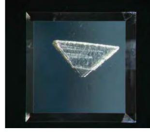
After a process of trial and error, the Stardust@Home team settled on this window as the optimal way to mount the pieces of the aerogel for study. In this configuration the "keystone" containing a candidate track is sandwiched between two silony nitride windows, each only 70 nanometers in thickness. Image: Regents of the University of California, Stardust@Home
