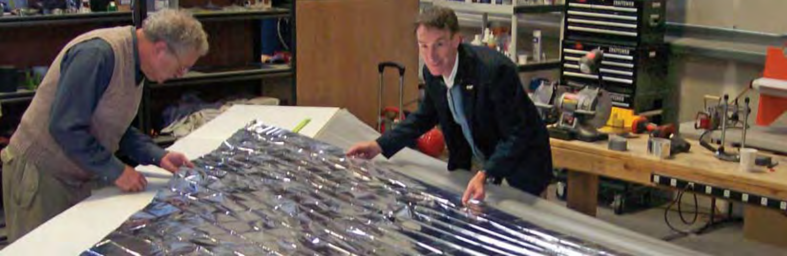
Above: Bill and Louis Friedman inspect the solar sail after it was deployed by hand (to test packing and folding) at the LightSail System Review Meeting, which was held in San Luis Obispo, California in December 2009.
