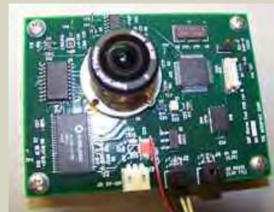
video cameras is shown above—they will be installed on the spacecraft engineering model (at the ends of two solar panels) for the mechanical tests. The Lumidyne Test Experiment sensors (nano-accelerometers) are undergoing testing in separate field experiments.
