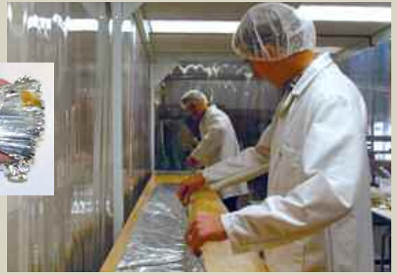
I also went into the clean room to inspect “my” solar sail. (To reassure those who know me, I don’t really handle flight hardware.) The sail material was supplied by the Orcon company and comes in rolls from which the actual sails are assembled by seaming material. Above, Stellar engineers Chris Biddy and Michael Bertino are folding the sail material in the very special way that permits smooth deployment in space. The folding of a single sail (inset) took about 20 hours.
