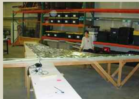
up a sail measuring about 5.6 x 5.6 meters with 4-meter booms. The mass-to-area ratio of LightSail-1 is 144 grams per square meter, the lowest of any solar sail spacecraft to date. For comparison, Cosmos 1 was 175 grams per square meter and IKAROS was approximately 787 grams per square meter. The lower the ratio, the greater the spacecraft’s acceleration.
