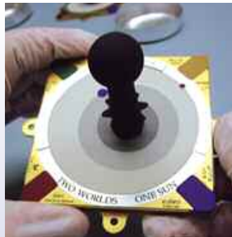
The Planetary Society's MarsDials, aside from their duties as calibration targets for the Panoramic Cameras on Spirit and Opportunity, have much to say to the Red Planet's future visitors. These before-and-after pictures show a MarsDial in the lab on Earth and, later, covered with the ruddy dust of Mars.
