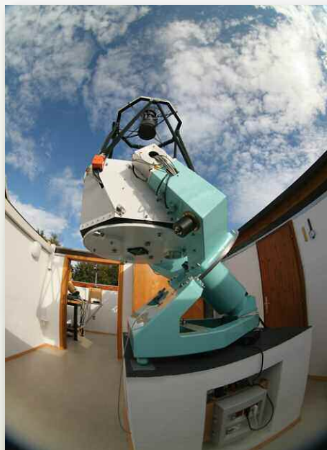
The 60-cm, robotically controlled Cichocki telescope used by Herman Mikuž at the Črni Vrh Observatory in Slovenia. Photo: Črni Vrh Observatory
