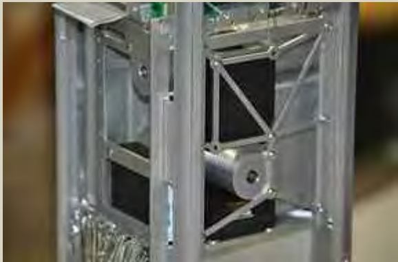
The cubesat module is pretty small, but it is large enough for our extremely small electronics. Shown here is the electronics compartment with two of the gyros visible. Gyros are used for attitude stability to point the spacecraft in the proper direction. Together with the onboard accelerometers (not shown), the gyros will provide complete information about the spacecraft’s position and velocity during flight. In the lower left of this figure, you can see the folded sail in its compartment.
