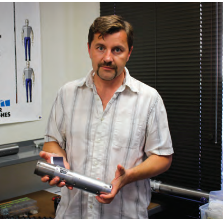
BELOW Kris Zacny, vice president and director of exploration technology for Honeybee Robotics, holds part of the instrument package for the Planetary Deep Drill, which contains a microscope capable of resolving particles that are only 0.5 microns across.
