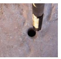
42 feet) below the surface. Though it was drilling, it was so deep that one could not actually hear the drilling sounds. During the drilling process, the PDD drills 10 to 20 centimeters over the course of tens of minutes, then the human crew reels it up from the hole, cleans out the cuttings, then lowers it again. This gets repeated over and over.
