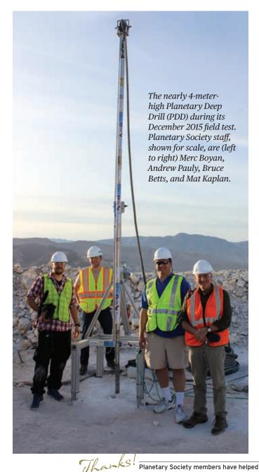
**NOTHING SAYS** "holiday season" like a 4-meter wireline drill digging its way into tens of meters of rock in a gypsum quarry. So, in December, several of us from The Planetary Society took a road trip to a gypsum mine near the Salton Sea in southeastern California. For several weeks in November and December 2015, the quarry was home to the first field test, sponsored in part by The Planetary Society, of the Honeybee Robotics Planetary Deep Drill (PDD).
