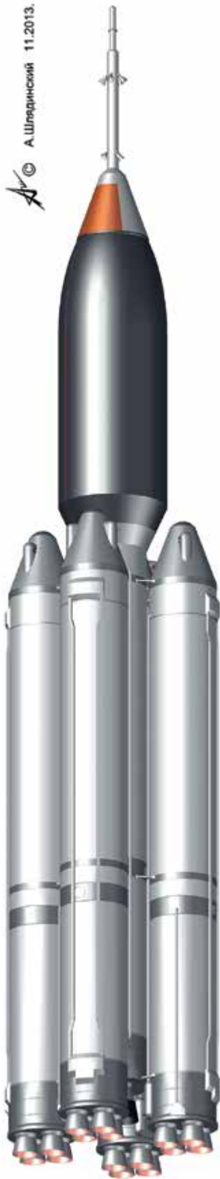
Variant of «Quark» with a load capacity of about 70 tons in low orbit
